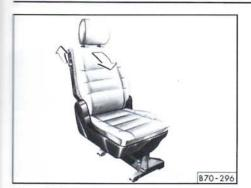
The single seat next to the centre seat bench can be folded, in such a manner, to enable easy access to the rear seat bench.
