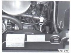
The engine must be running at idling speed, the handbrake must be applied and the selector lever at "N".
