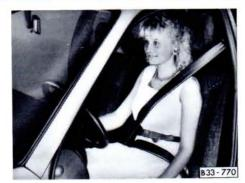
The shoulder part of belt must run roughly across the centre of the shoulder as shown – on no account against the neck – and be firmly in contact with the body.
