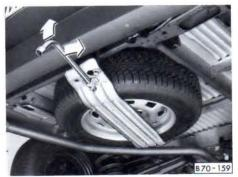
■ Remove securing screw A completely. The spare wheel carrier then rests on the safety screw B.
