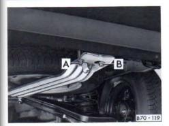
The spare wheel is secured under the rear of the vehicle in a special hinged carrier.
