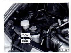
The reservoir is located in the engine compartment on the right looking forward.
