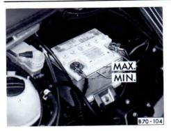
The battery is in the engine compartment on the left looking forward. It can be reached when the lid of the battery box is removed.
