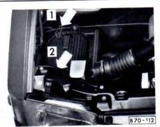
The paper filter element in the air cleaner is normally renewed as detailed in the Service Schedule. In very dusty conditions the element must be cleaned or renewed at shorter intervals.
