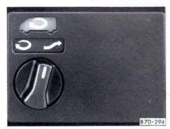
This switch can be used to change over to recirculating air. This will prevent badly contaminated air from entering the vehicle, e.g. when driving through a tunnel.
