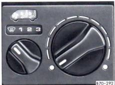
On vehicles with an air conditioner temperature regulation for the additional heater is by way of a rotary control on the right adjacent to the blower switch (centre illustration).
