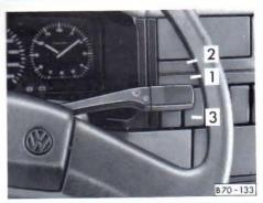
Wipers and washers only work when ignition is switched on.
