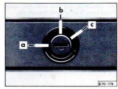
To unlock the tailgate or wing door insert key and turn it to right (c). Hold in this position and press button in.
