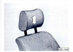
The front head restraints are adjustable for rake and height and should be set to suit the size of the person in the seat. Correctly adjusted head restraints together with the seat belts offer effective protection.
