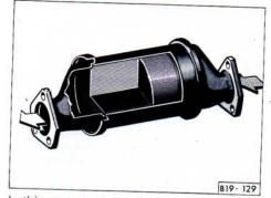
In this process three pollutants (three-way catalytic converter) are converted as follows.
