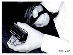
**To lengthen belt** hold the tongue at right angles to belt and pull belt through to the required length – see illustration.
