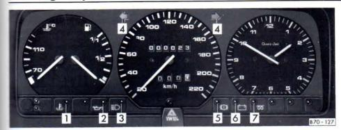
The layout of the warning lamps depends on the model and the engine fitted. The symbols shown here are also on the actual warning lamps.
