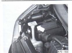
The fluid container is on the right of the engine compartment. The container holds about 5 litres, on vehicles with headlight washer system\* about 7 litres.
