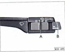
By repeatedly pressing button B in the windscreen wiper lever with the ignition switched on, the additional information is displayed, starting with the time.
