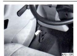
**To release** lock, pull lever on left under instrument panel until bonnet springs up slightly.
