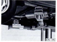
Short wheelbase vehicles, when unladen can as an exception be lifted on a single column hoist.
