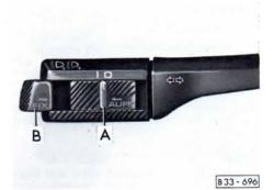
The system is operated with the sliding switch A and the press button B on the turn signal lever.
