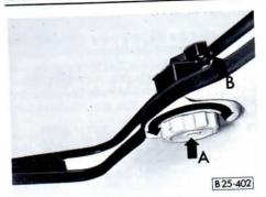
The roof is opened and closed with the hand-wheel.
