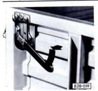
To lower the dropsides pull locking handle outwards until the pin is clear of retaining hole then swing handle down.
