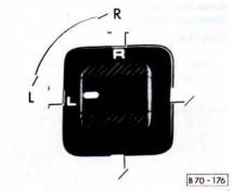
**Electrically adjustable mirrors\*** are set by moving the knob in the driver's door trim.
