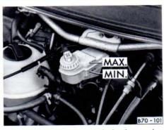
The brake fluid reservoir is in the engine compartment.
