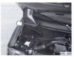
**To close** bonnet lift it slightly adn pull the strut forward – see illustration. Let bonnet drop into locks from a height of about 30 cm – do not press it closed.
