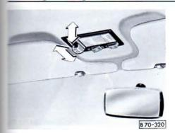
With ignition switched on, the roof can be spened and closed with switch.
