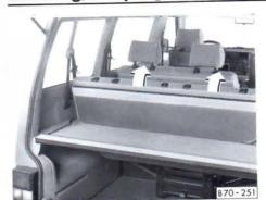
The rear seat backrest with a loading/sleeping surface can be folded forward to provide a large loading and/or sleeping surface.
